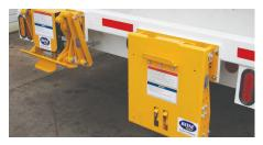
Add Bayne Thinline<sup>®</sup> Premium Cart Tippers Outfit your truck with a single or dual Bayne Thinline<sup>®</sup> premium mobile lifters and reduce the stress and strain on personnel who manually load the vehicle, and increase route efficiency.
