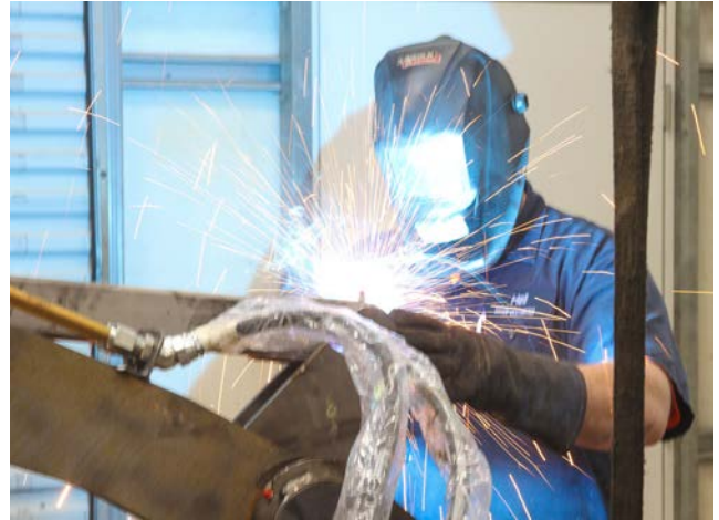
Weldments, cylinders, and valves are reconstructed and tested by Heil® certified technicians to ensure that OEM specs are met.
