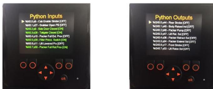
By verifying that each one of these inputs are correct on the InSight display, the technician can often locate the problem before ever checking the hydraulics or disconnecting electrical connections.
