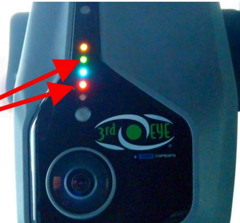
Look at the 4th light from the top. This is an orange indicator light for cellular connection. Is it on and solid orange? If so, this indicates your cellular connection is good and connected to the 3rd Eye portal.
