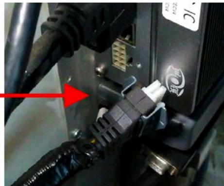
Then reconnect the connector and restart the system by turning on the key switch and allowing the Gateway to boot up which can take up to 5 minutes. Once the Gateway boots up, look at the window unit. Notice if
