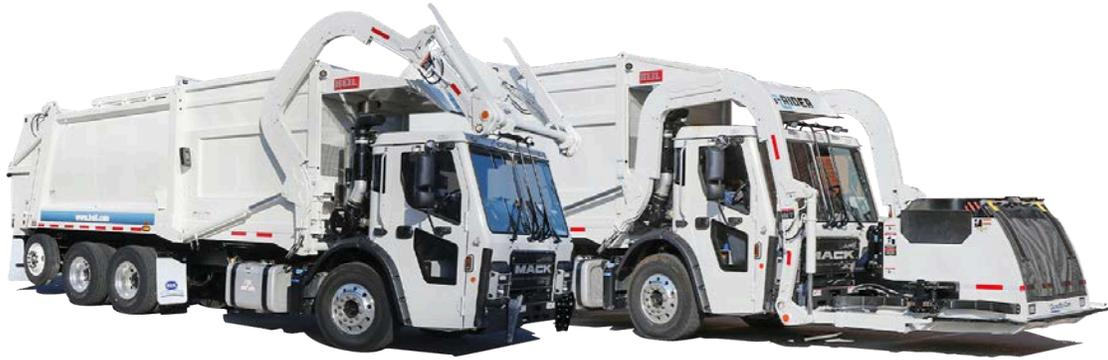
Some haulers use HEIL Automated Front Loaders (AFL) to collect residential routes. Typically, these are not set up to collect commercial dumpsters; instead, they have a Curotto-Can attached to the forks along with hydraulic and electrical connections to complete the working attachment.
