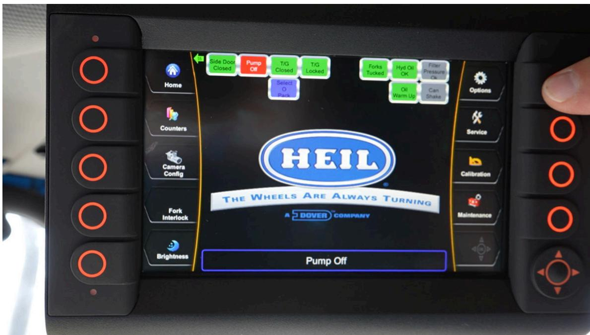
Then press the "Options" button. This will prompt you to provide the password for the display. After entering the password, press the OK button.
