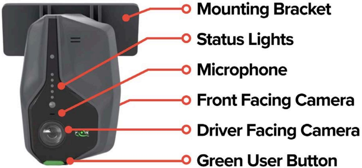
The Window Unit consists of a driver-facing camera, a front-facing camera, a microphone, a green user button, and LED lights used for troubleshooting. The LED lights are important in understanding what is happening with the 3rd Eye Gateway. The user button at the bottom of the Window Unit initiates a 12-second video event. The Window Unit is attached to the front windshield using a replaceable mounting bracket, part number 3EC-V4WUBRACKET.
