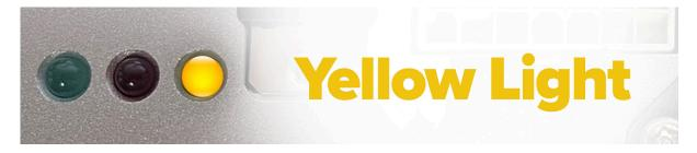
**YELLOW LIGHT** – The yellow light has three statuses. When illuminated, it indicates that the battery is charging. When not illuminated, it shows the battery is fully charged. When blinking, it signifies that the battery has failed or is no longer detected by the V4 Gateway.
