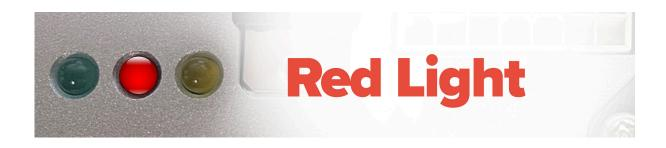
**RED LIGHT** – When the ignition switch is turned on, the red light will begin to blink. This indicates that the V4 Gateway is booting up. This status will persist until the V4 Gateway has fully booted up. Once it is fully booted, the light will turn solid red instead of blinking, indicating that the V4 Gateway is fully booted up. After the V4 Gateway has finished booting up, the window unit will then begin its boot process.
