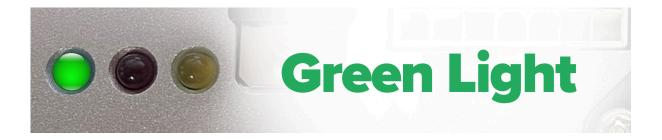
**GREEN LIGHT -** When illuminated, it confirms that the connection to the chassis battery is present. When not illuminated, it indicates that the battery connection is either absent or that the fuse has failed. In either case, we would troubleshoot a disconnect from the chassis battery.
