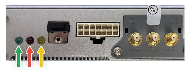
There are three lights located on the 3rd Eye V4 Gateway: green, red, and yellow. The status of the V4 Gateway can be determined by the status of these lights.
