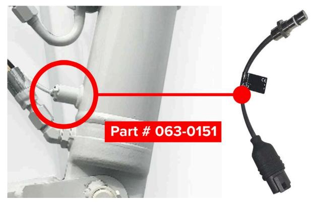
The proximity switch cable has a three-pin connection, and the wire colors are Brown (12V power), Blue (ground), and Black (signal). In the Heil harness connecting to the proximity switch connector, you will find Black (12V power), White (ground), and Orange (signal). These proximity switches detect the hydraulic cylinder piston.
