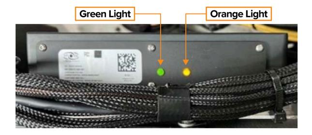
When the power is turned on, both the green and orange lights turn on for a few seconds. Then the orange light turns off, and the green light blinks.
